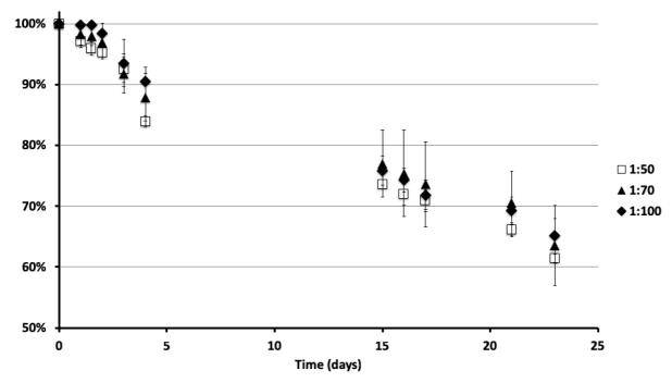
**Figure S2.** Time evolution of the area of  $G/TA_x$  matrixes incubated in citrate/phosphate buffer pH = 7 at room temperature. One could note the shrinking over the time period. There is no difference in the three different G/TA molecular ratios tested.
